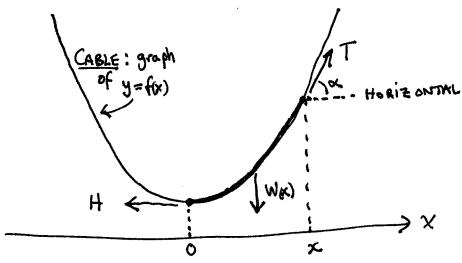
Q3(b). Combine the previous two equations, and remember some Calc I, to get the Cable Equation:
