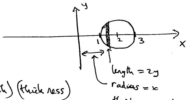
$$Vol = \int 2\pi (\text{radius}) (\text{length}) (\text{thickness})$$
