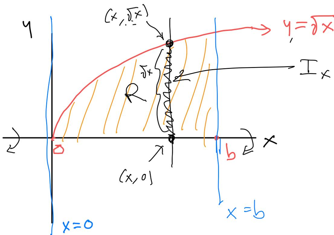
rotate  $I_x$  around  $x$ -axis to get a disk of radius  $\sqrt{x}$ .
