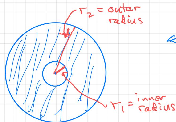
$$\text{washer area} = \pi r_2^2 - \pi r_1^2$$
